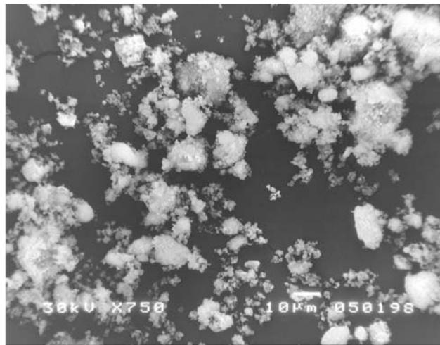
Figure 2. Characteristic microstructures of hydrothermally obtained hydroxyapatite
